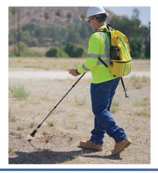
The Inspectra Max is an accurate methane analyzer with full traceability. Sensitive to below 1ppm, this model offers all the advantages of optical detection in a highly compact and portable device. With precise and reliable methane readings that can follow planned routes, operators can view results on a smartphone via Bluetooth connection to an integrated data platform.
